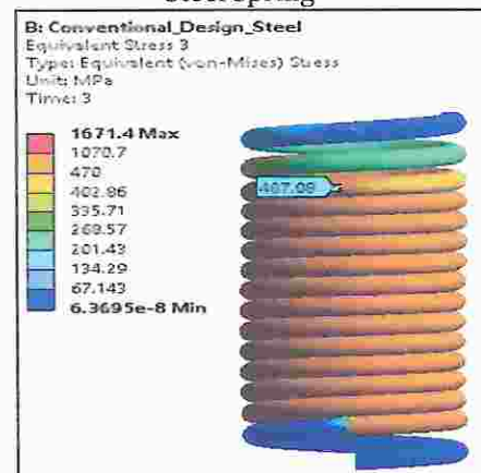
Figure.6 Stress Plot Load Case 3 Related to Steel Spring
